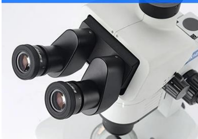
5~45° Tilting Trinocular Head & PL10x/23mm Eyepiece
